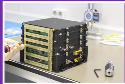
SO/PHI E-UNIT QM model during assembly phase.
