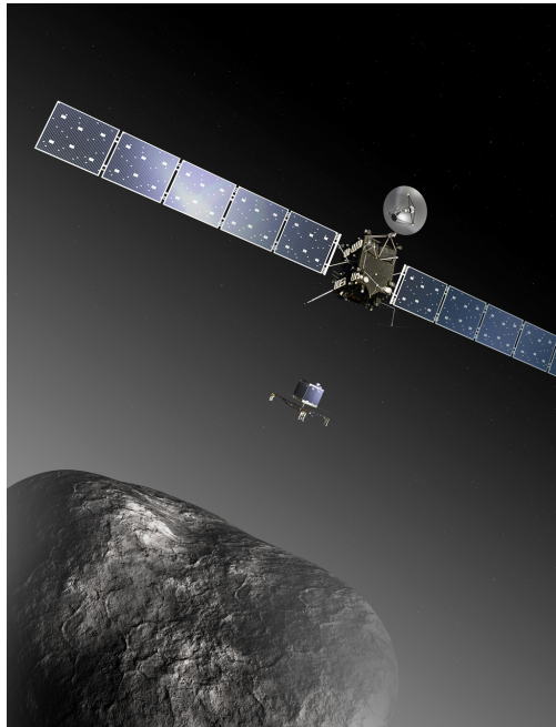
Figure 1.9: Rosetta and Philae at the comet. Artist's impression of the Rosetta orbiter and the Philae lander to 67P/C-G. The image is not to scale; Rosetta spacecraft measures \sim 32 m, while the comet nucleus is estimated to be about 4 km wide. The image has been extracted from the Rosetta-ESA web page http://www.esa.int/Our_Activities/Space_Science/Rosetta . Under the copyright of: ESA-C. Carreau/ATG mediala.
