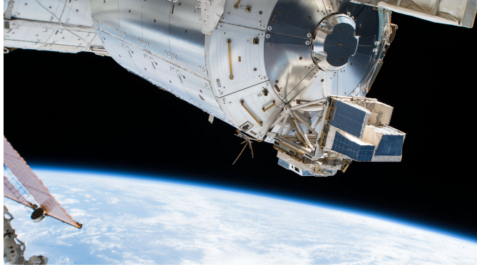
Figure 2.3. Real image of the ASIM module on the Columbus Externals Payloads Adaptor (CEPA) of the ISS.
