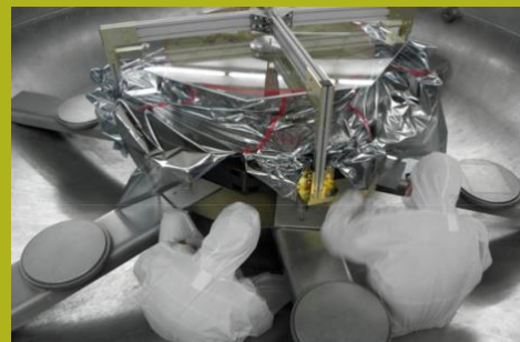
Sunrise telescope mirror aluminizing at Calar Alto observatory
