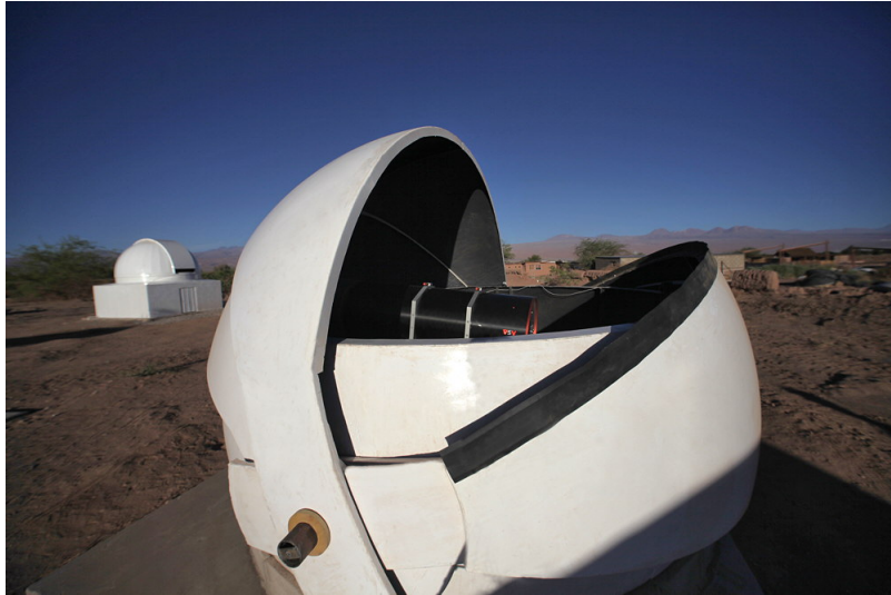
Figure 33: ASH2 is a 0.40 m (f/3.7) diameter remotely controlled telescope. Credits: Nicolás F. Morales Palomino.
