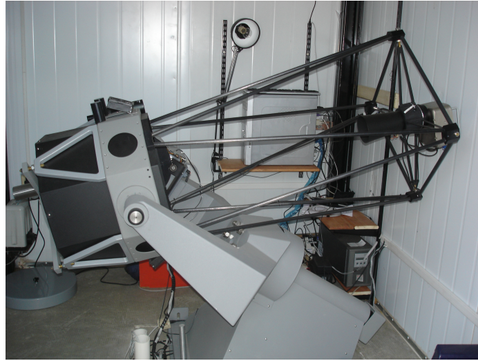
Figure 31: ASH is a 0.45 m (f/2.8) diameter remotely controlled telescope. Credits: Nicolás F. Morales Palomino.
