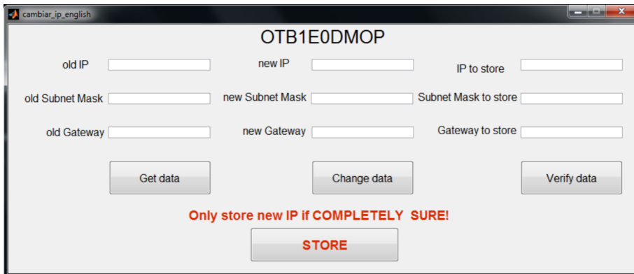
Figure 5.3: Graphical user interface to remotely change the IP address of the automaton
