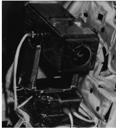
Figure 1.6: NASA space shuttle’s sensitive payload bay monochrome video cameras to record the Earth’s nighttime lightning activity ( Boeck and Vaughan Jr. , 1990)
