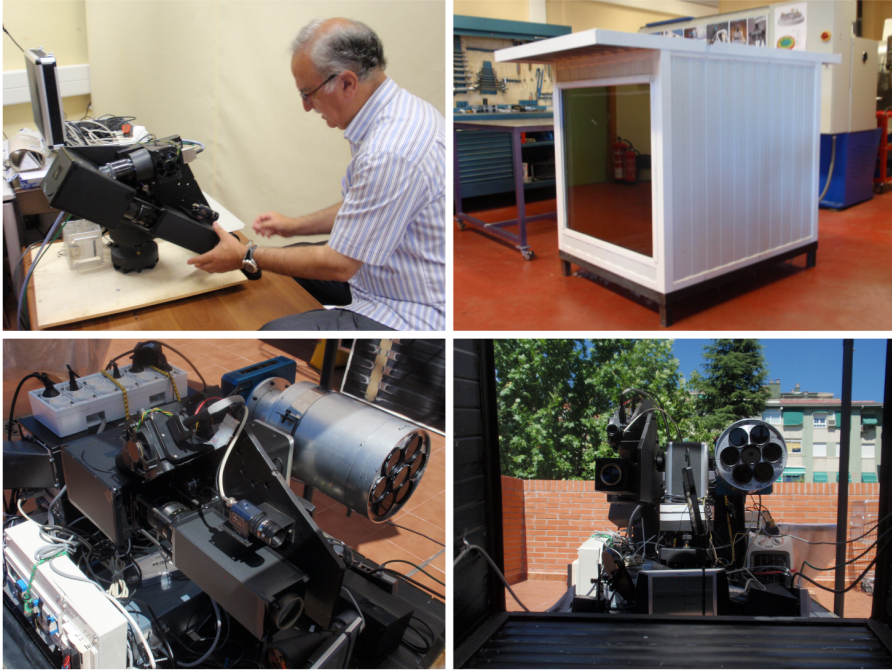
Figure 2.11: GRASSP v1.x housing images. Up-left: Justo Sánchez del Río installing the spectrograph on the telescope mount at the Instituto de Astrofísica de Andalucía (IAA) dependencies. Up-right: GRASSP v1.x housing at the IAA workshop. Bottom-left and right: GRASSP v1.x inner subsystems
