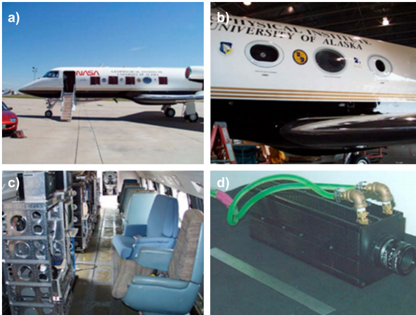
Figure 1.18: EXL98 Gulfstream II aircraft and NIR camera. (a) The aircraft, with the specialized windows covered for protection when not in flight. (b) Two of the quartz windows. In the left window the Color, Wide field of view (FOV) and Narrow FOV cameras are mounted and in the right window the NIR and NUV imagers. The center window is the standard Gulfstream Plexiglass. (c) The interior of the aircraft; observations could only be made out of the left-hand side. (d) The NIR imaging camera ( Siefring et al. , 2010)
